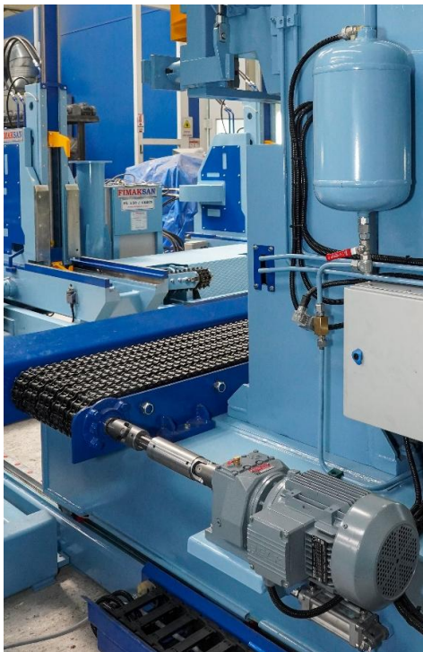
Sawn board & sawdust Removal chain
