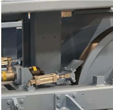
*Automatic sawdust scraper and blade diesel sprayer feature
