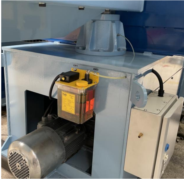
*Auto Lubrication Unit
