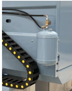
*Automatic sawdust scraper and blade diesel sprayer feature
