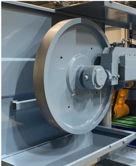
*Solid flywheel, wide flywheel surface
